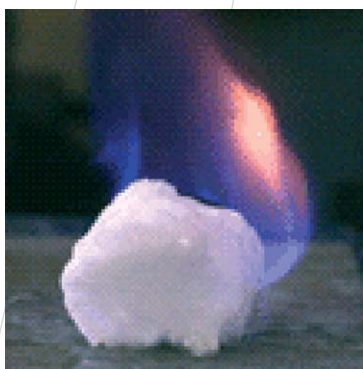
Figure 43. Methane hydrate structure, drilling core samples and combustion experiment
